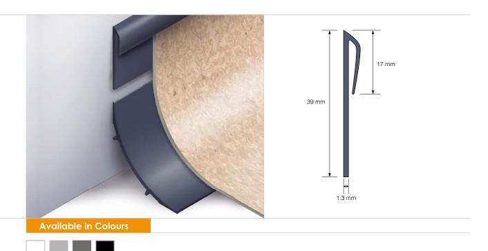
A flexible PVC capping strip to be fitted along the top of floor coverings when coving up the wall. To be used in conjunction with GCF-038 and adhered to the wall using Grabfast Gold.
